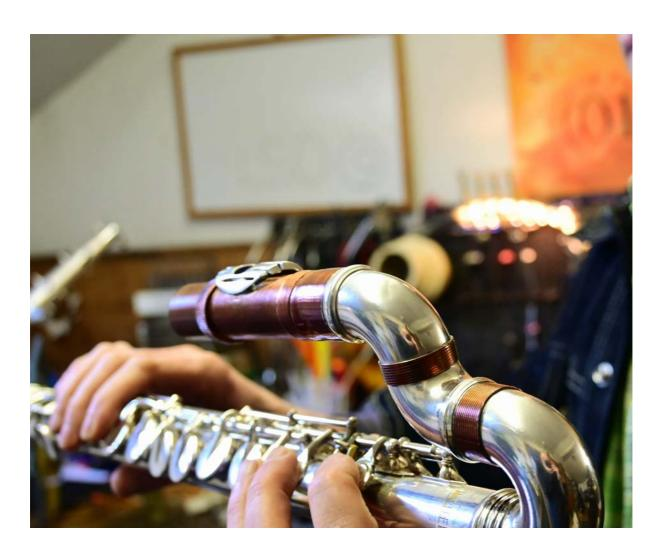
... arriving now at the mouthpiece; ; clark tech modifications have resulted in replacing the smooth mouthpiece — head joint connector; ; with a threaded connector; ; as was also done in the connection between the neck joint and the body of the flute; ; the result of which gives an internal threaded and external 'sandwich '/ 'echo chamber 'type of construction; ; where threaded cooper tubing is encased within an outside copper [or silver] shell...
