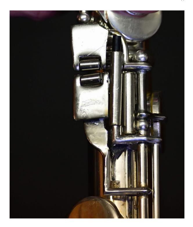
1] improved overall positioning of the keys / key pad ;; utilization of an optimal roller - roller - roller corner configuration;; and tight tolerance close key abutment . . .
