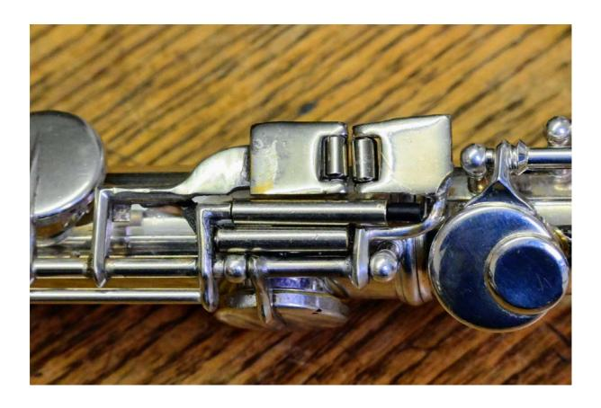
2] flat key padlet surfaces for the d sharp / e flat and c sharp / d flat keys; ; used to increase finger efficiency and positioning friendliness; ; along with additional key weighting response . . .
