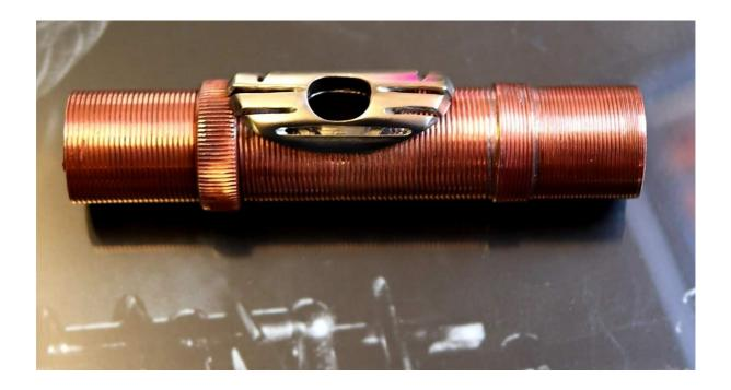
... the final mouth piece sections; including the external resonating chamber and the additional threaded copper sleeves and resonating discs; as a consummate work for engineering and machining expertise; were turned by john entwhistle on a conventional manual lathe; without the use of any drawing or sketch and done during the course only a few shop sessions; with additional resonating discs being stamped out on a genuine old style fly press; and were also executed by hand...
